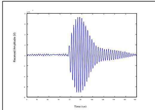
Figure 4. Pulse-echo test with a large cMUT device in air. Excitation of the 100V biased transducer with one 200V unipolar pulse. The received signal was filtered with a 30 kHz high-pass filter and amplified 40 dB. Target: a 250x450x1 mm steel plate placed 100 cm from the transducer. The received signal was averaged 64 times.
