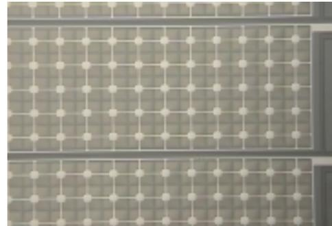
Fig.2. Close view of a 128 element array of  $36\mu\text{m} \times 36\mu\text{m}$  cMUTs with a  $0.34\mu\text{m}$  thick silicon membrane.
